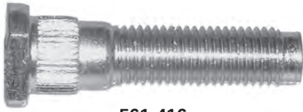
561-416 M12 x 1.5 x 52mm Knurl diameter: 14.8mm
