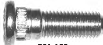
561-139 M12 x 1.5 x 37mm Knurl diameter: 14mm (Code M.3.0)
