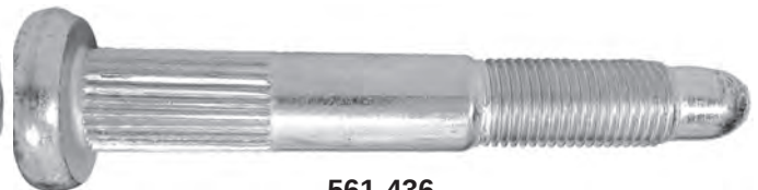
561-436 M14 x 1.5 x 104mm Knurl diameter: 16mm
