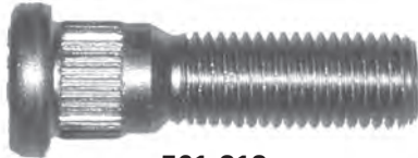
561-312 M12 x 1.5 x 44.4mm Knurl diameter: 14.17mm
