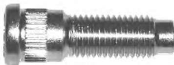
561-248 M12 x 1.5 x 43mm Knurl diameter: 14.5mm (Code Fm1)
