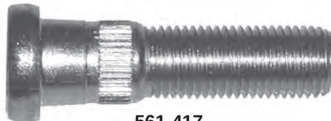
561-417 M14 x 1.5 x 54mm Knurl diameter: 15.7mm (Code DK)
