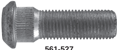
561-527 M14 x 1.5 x 45.5mm Knurl diameter: 16.5mm
