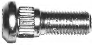
560-386 7/16-20R x 1-5/16" Knurl diameter: .555 (Code: DN)
