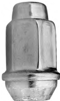
558-094 1/2-20R 3/4" Hex 1-39/64" Height Stainless Steel Capped
