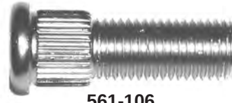
561-106 M12 x 1.5 x 38.5mm Knurl diameter: 14.7mm (Code M.2.0)
