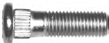
561-169 M12 x 1.5 x 43mm Knurl diameter: 12.85mm (Code CI)
