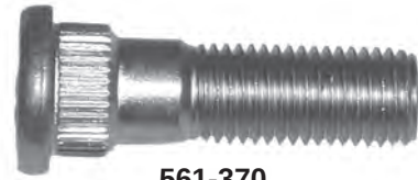
561-370 M12 x 1.5 x 44mm Knurl diameter: 15.8mm
