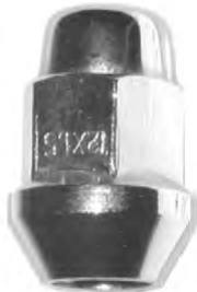
559-077 M12 x 1.5 Acorn Bulge 19mm (3/4") Hex 35mm Height Cone Angle: 60° Chrome
