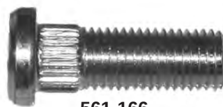
561-166 M12 x 1.5 x 32mm Knurl diameter: 13mm (Code M.3.5)
