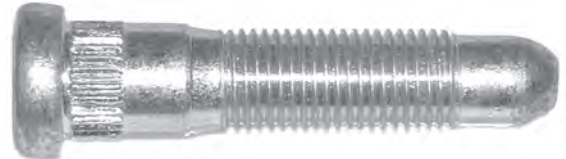
561-428 M14 x 1.5 x 65mm Knurl diameter: 15.7mm
