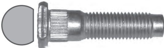
561-376 M12 x 1.5 x 49mm Knurl diameter: 13.9mm
