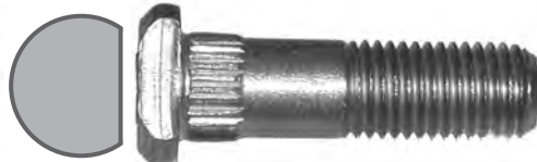
561-309 M12 x 1.5 x 42.7mm Knurl diameter: 13.08mm
