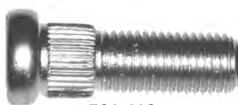
561-112 M12 x 1.5 x 40mm Knurl diameter: 12.5mm (Code M.4.6)
