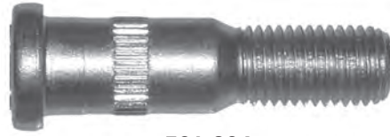
561-264 M12 x 1.5 x 52.6mm Knurl diameter: 14.33mm
