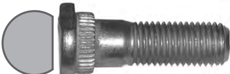
561-361 M12 x 1.5 x 41.0mm Knurl diameter: 16.5mm
