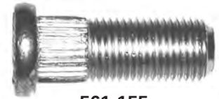
561-155 M12 x 1.25 x 33mm Knurl diameter: .12mm (Code: H.1.0)
