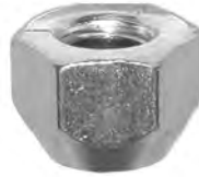
559-172 M12 x 1.5 21mm (13/16") Hex 18mm Height Cone Angle: 60° - Zinc
