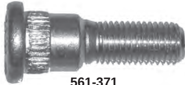
561-371 M12 x 1.5 x 43.8mm Knurl diameter: 17mm
