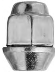
558-124 1/2-20R 13/16" Hex 1-9/32" Height Stainless Steel Capped
