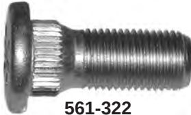
561-322 M12 x 1.25 x 30.2mm Knurl diameter: 14.27mm
