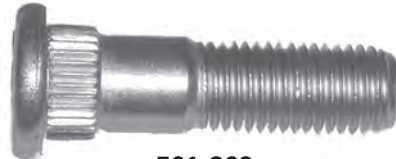
561-369 M12 x 1.5 x 46mm Knurl diameter: 15mm
