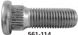
561-114 M12 x 1.5 x 38mm Knurl diameter: 14.35mm (Code C.U.1)
