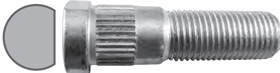
561-502 M14 x 1.5 x 50mm Knurl diameter: 16.02mm
