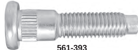
561-393 M12 x 1.75 x 55mm Knurl diameter: 14.6mm
