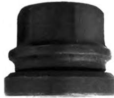
559-196 M14R x 2.0 21mm Hex 22.6mm Height 29.8mm Seat - Black
