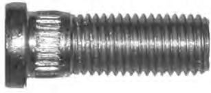
561-115 M12 x 1.5 x 35mm Knurl diameter: 12.7mm
